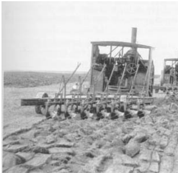
Figure 5: Two Marshall gas tractors" (35-70HP) breaking sod on the Canadian Wheatlands Company Limited holdings near Suffield, in 1913 (Glenbow Archives, NA-587-8).
