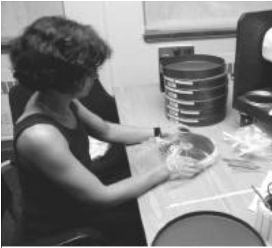
Preparation for the move of acetate-base films in a state of deterioration. A film is placed in a plastic bag with molecular sieve to absorb acid vapors. The bag is then sealed and put in a container with the film.
