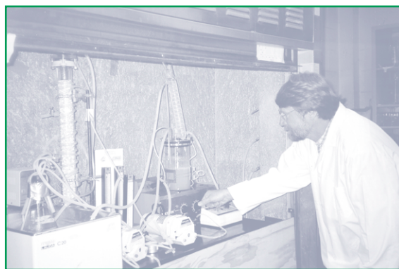
Dr. Andrew Daugulis, professor of chemical engineering at Queen's University, adjusts the parameters on a bench-scale Two-Phase Partitioning Bioreactor used to clean contaminated soil.
