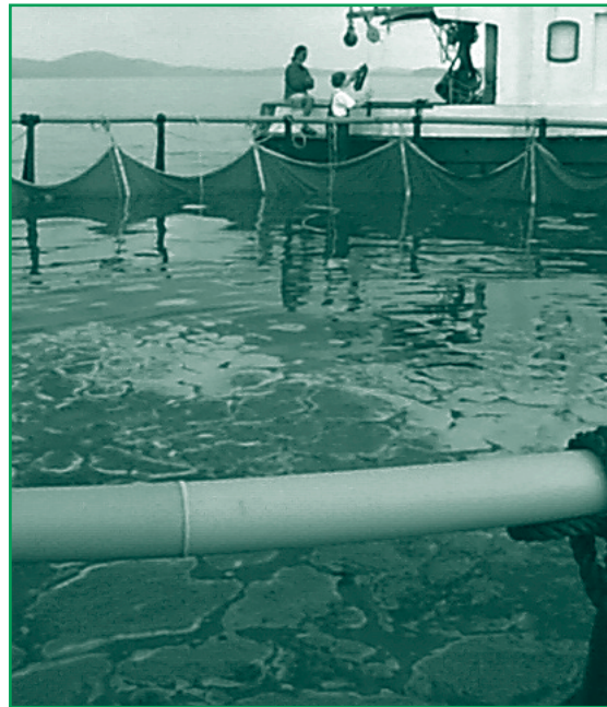
Dye is added to the pesticide solution in a salmon aquaculture net pen so that when the tarp around the enclosure is removed, scientists will be able to track the dispersing plumes and determine their toxicity.
