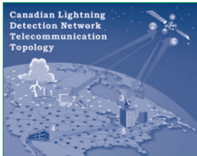
1) Canadian Lightning Detection Network sensors pick up the electromagnetic signal from a lightning stroke, and 2) the signal data are uplinked to a communications satellite, 3) downlinked to the Telesat Hub in Toronto, and then 4) relayed to the Network Control Centre (NCC) in Tucson, where they are integrated with other data. 5) Solutions are relayed from the NCC back to the Telesat Hub in Toronto, 6) uplinked to the satellite, and 7) broadcast to the users' workstations.
