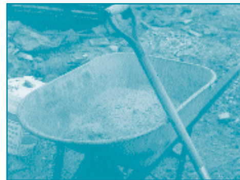
Daily Manual Ash Removal from a Small BCS
