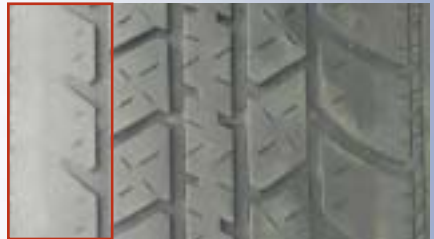
Uneven tread wear can be caused by improper wheel alignment or a tire imbalance.
