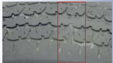
A tire must be replaced when the tread wears even with the treadwear indicator.
