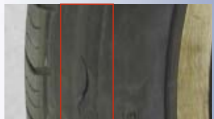
Tires with cuts, cracks, or bulges in the sidewall or in the tread should be replaced.
