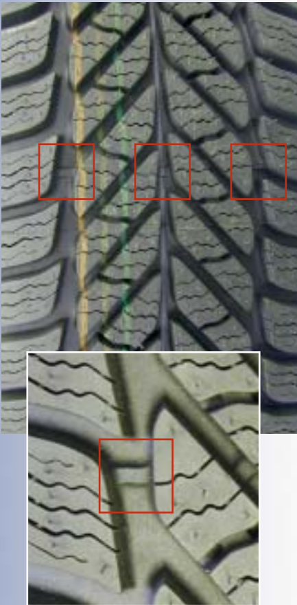
The treadwear indicator marks the minimum allowable tread depth.
