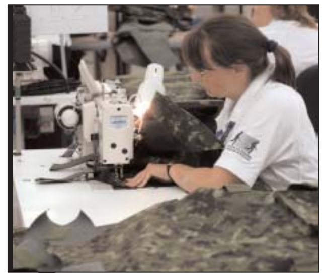
A woman sews a fragmentation protective vest in a manufacture in Arnprior, Ont.
