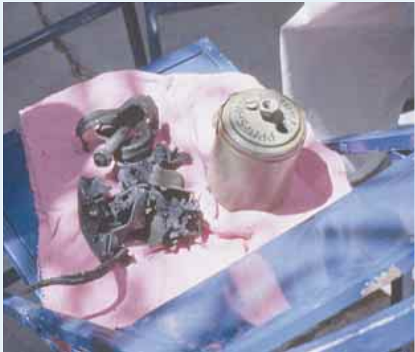
A POM-Z bounding mine before and after destruction.
