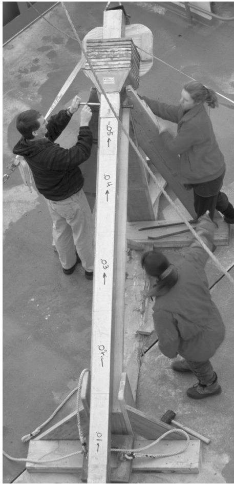
Figure 2 Kasten core on deck before being taken to the on-board laboratory for analysis.
