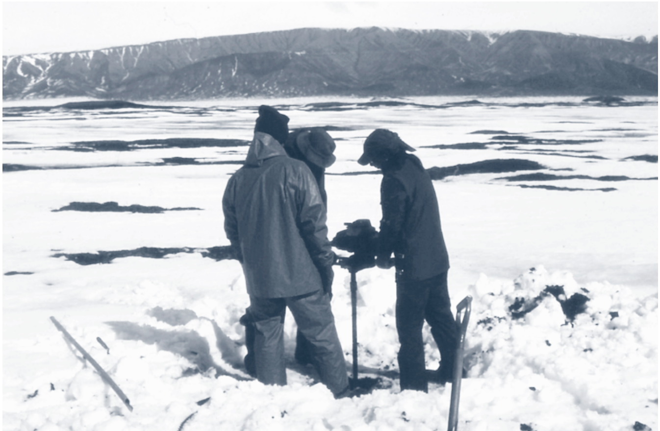
Figure 5 Collecting a permafrost sediment core. The corer was custom built by Michel Allard (Université Laval), supervising (left), and is being operated by Daniel Fortier (to left) and Isabelle Duclos (to right). Photo: C. Ellis.
