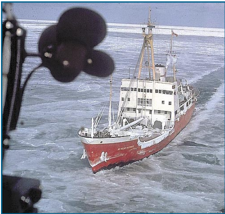
Photo 1.8: Coast Guard buoy tender/icebreaker escorts small freighter through rafted new and grey ice
