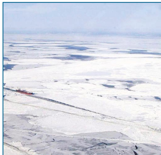
Photo 2.9: Ship moving through very close pack grey-white ice and patches of nilas.
