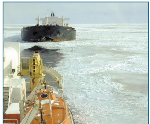
Photo 3.1: Escorting an oil tanker through very close pack, heavily rafted grey ice.
