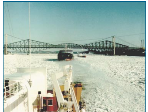
Photo 3.2: An icebreaker escorting a freighter above the Québec City bridges clearly show thick river brash ice.
