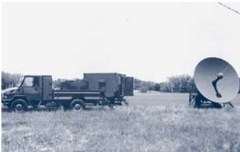
Tactical long-range communication terminal (TLRCT) in the field
