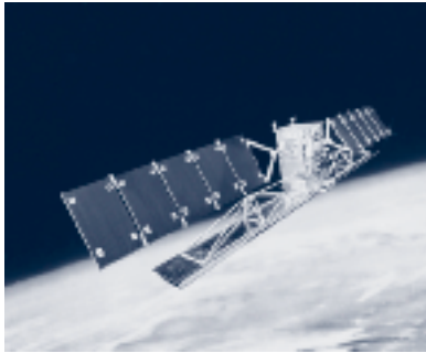
RADARSAT-1 Earth observation satellite, launched in November 1995, uses a powerful microwave Synthetic Aperture Radar (SAR) system to collect imagery of the Earth day or night and in all weather conditions.
