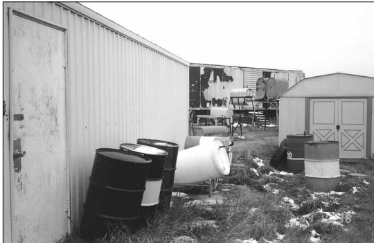
Barrels kept on the grass without any secondary containment at CFB Cold Lake. From the Auditor General's 1999 Report, Chapter 13, National Defence – Hazardous Materials: Managing Risks to Employees and the Environment.
