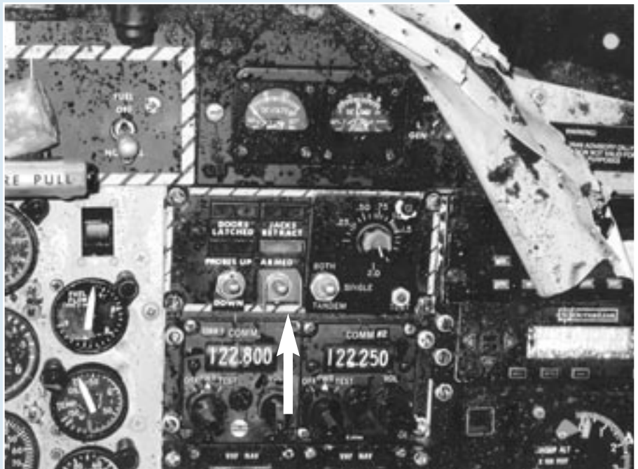
System indicating lights and door armed switch (indicated by white arrow) in the ON position
