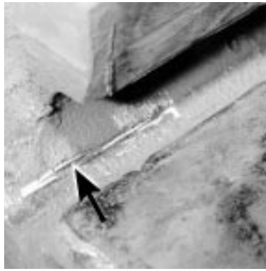
The casting defect after some exploratory work with a die grinder exposing a possible crack (arrow).
