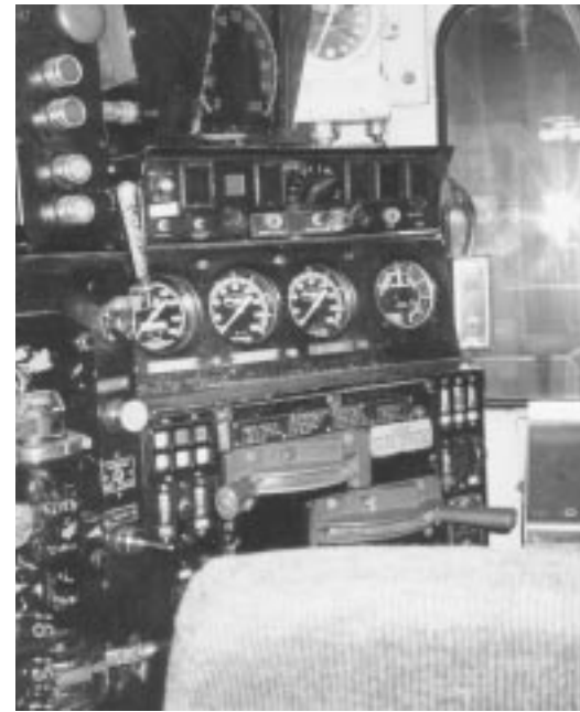
Control stand in the locomotive engineer's operating compartment of a QNS&L locomotive.
