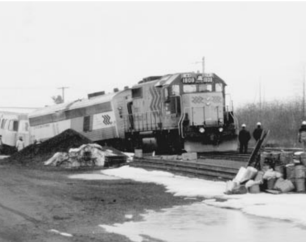
The damaged switch caused the locomotive, the electrical power unit, and three of the four coaches to derail.
