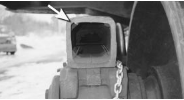
The fracture surface as found. The small shiny areas (arrow) and the light orange colour indicate that the fracture is relatively fresh.
