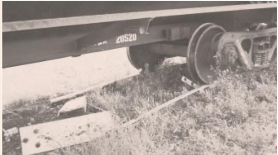
Trailing truck of the leading car at the damaged stop block.
