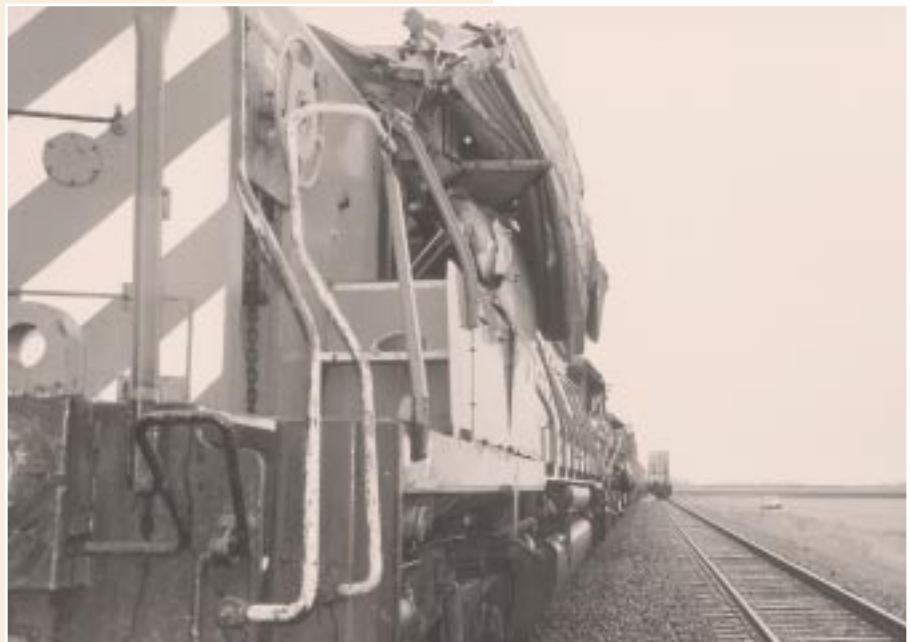
Wreckage of container from train 471 embedded in cab of lead locomotive of train 472.
