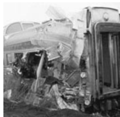
Damage to Skyline car due to contact with the foundation wall of the farm supply building.
