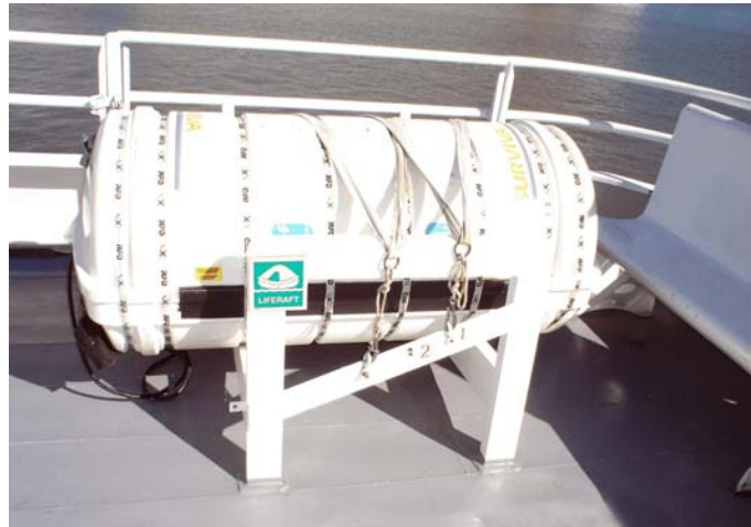
Photo 9. Liferaft secured by lashings fitted with senhouse slips
