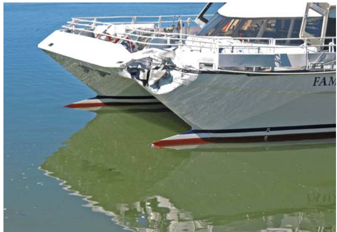
Photo 2. Damage to the port bow
