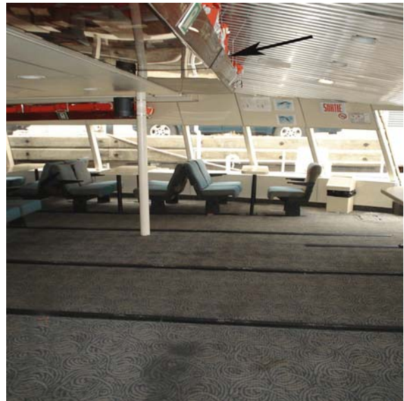
Photo 8. View of children's lifejackets (arrow) stowed in an overhead athwartships rack and rows of seats removed from the deck
