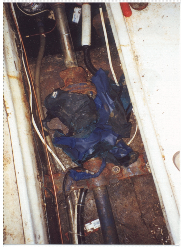
Photo 4. Remnants of the owner/operator's rain pants entangled in the shaft coupling and shaft.
