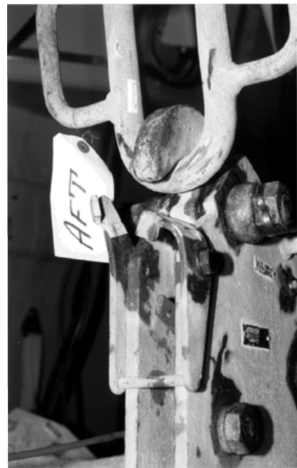
Photograph 16. Damage to the after retaining latch
