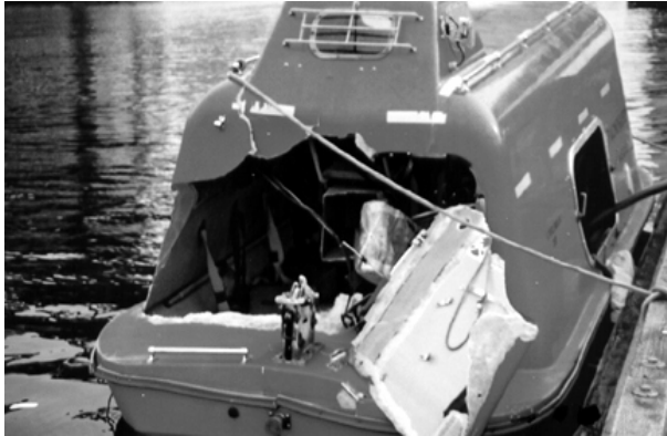
Photograph 14. Damage to the stern of the lifeboat
