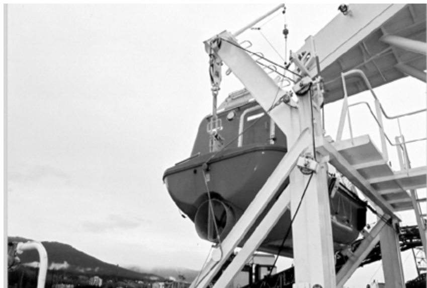
Photograph 6. After view of lifeboat, showing davit, gripe arrangement around bollards, suspension ring, hook, and hatch
