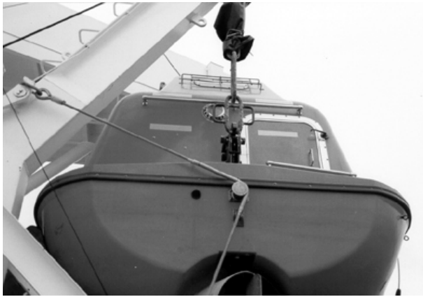
Photograph 7. After bollard, gripe, and hooked lever on davit
