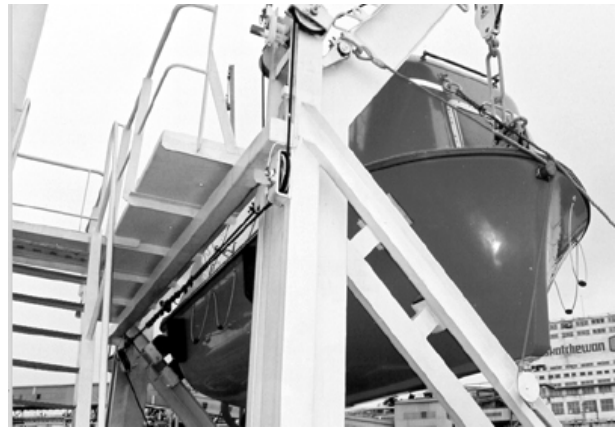
Photograph 8. Forward view of lifeboat, showing davit, gripe arrangement around bollards, suspension ring, hook, and hatch
