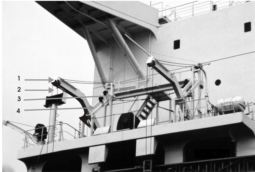
Photograph 3. 1. Davit, 2. Falls, 3. Embarkation platform, 4. Frame
