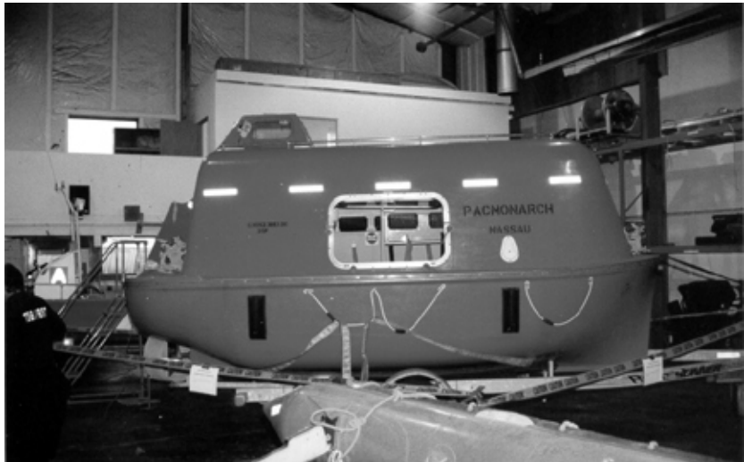
Photograph 2. Entry hatch and inboard side of lifeboat
