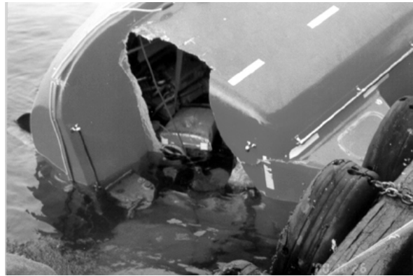
Photograph 15. Damage to the stern of the lifeboat
