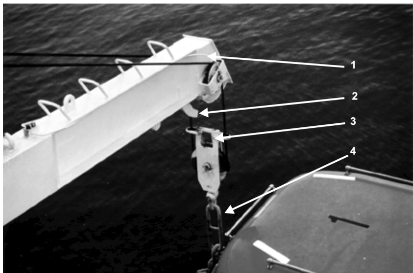
Photograph 4. 1. Davit head, 2. Horn, 3. Eye in floating block, 4. Suspension ring
