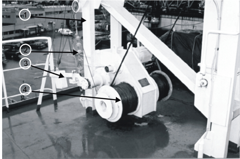
Photograph 5. 1. Frame, 2. Gripe, 3. Dead man's handle (winch brake), 4. Winch drum
