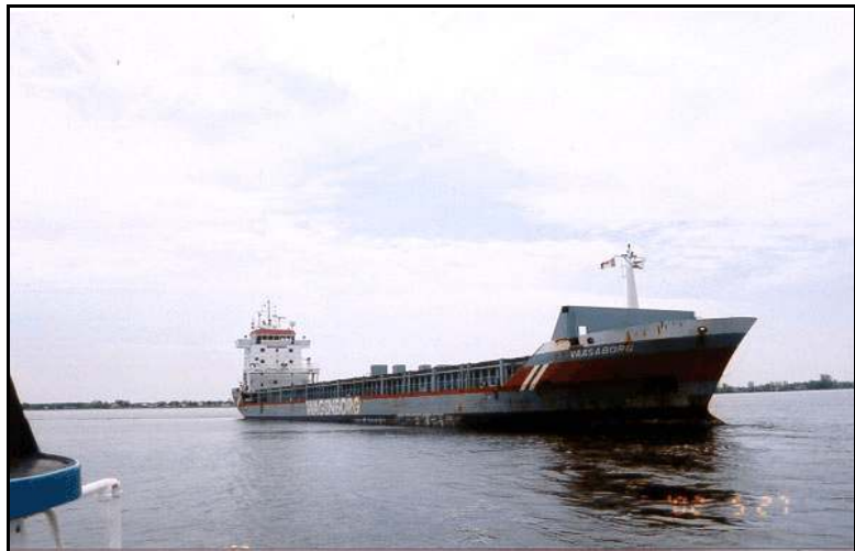
Photo 1. Vaasaborg aground. The vessel was refloated after lightening the cargo by some 1800 metric tons.
