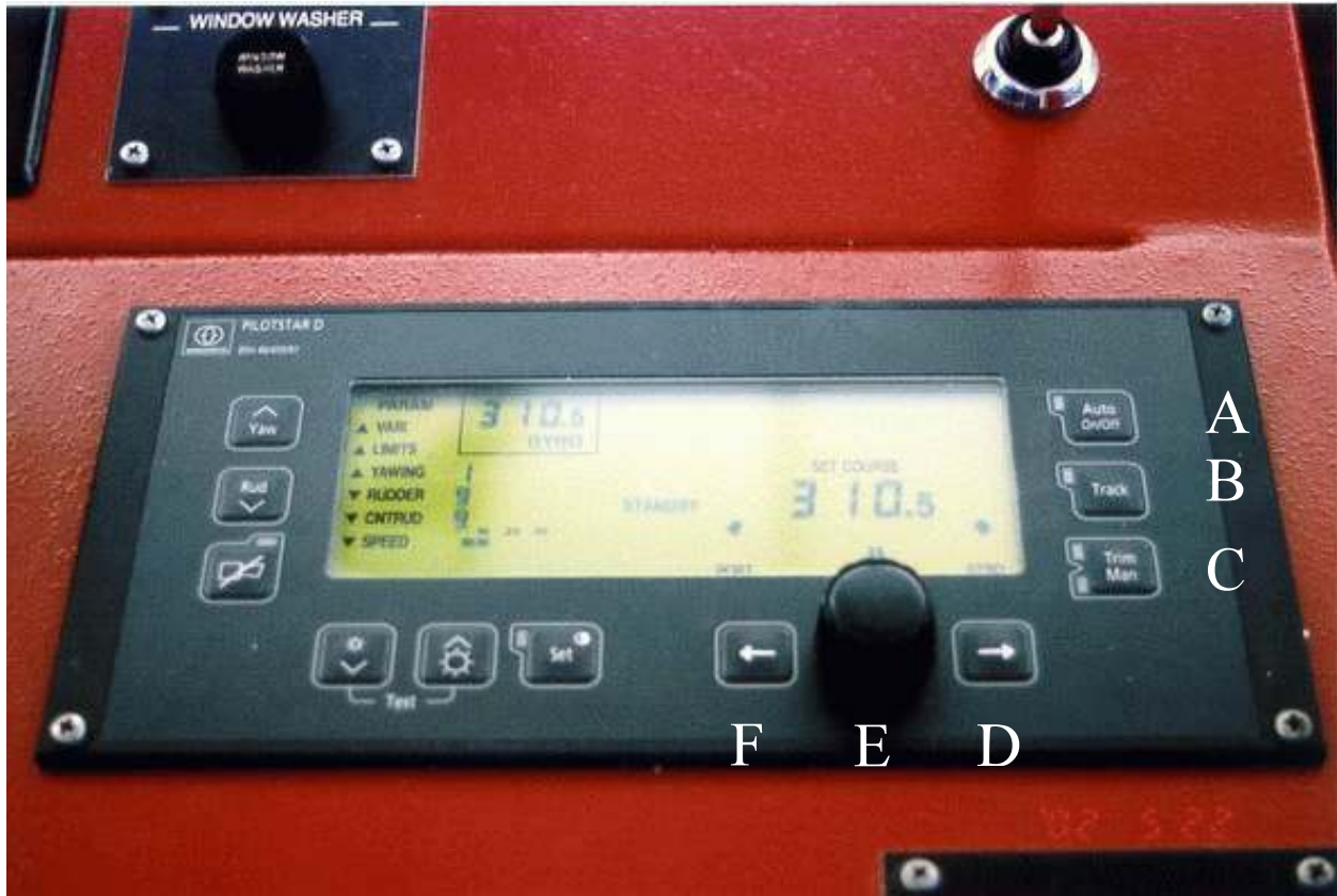
Photo 2. Autopilot control panel
