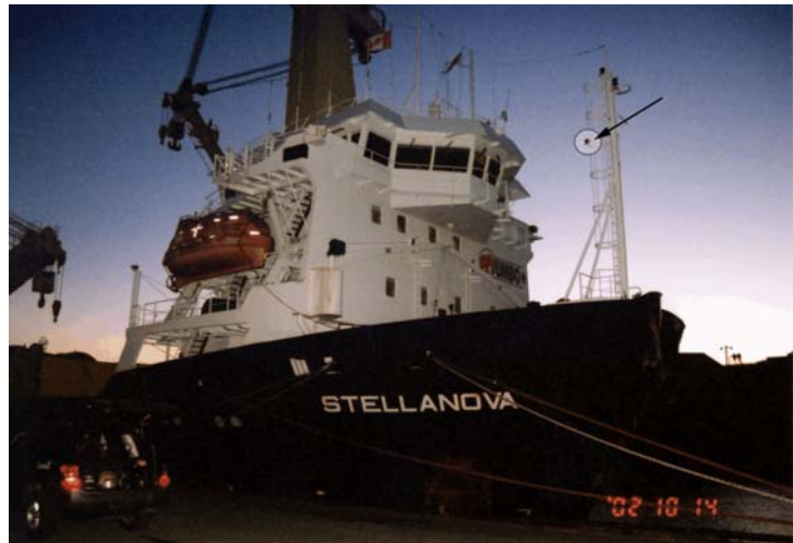
Photo 3. View forward from the bridge showing position of the blue steering light
