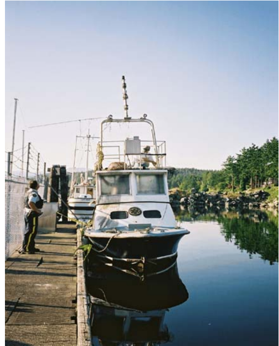
Photo 2. Bruce Brown , 2002. Note the addition of an enclosed wheelhouse, upper control station, and mast arch.
