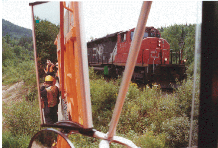
Figure 2—Visibility from a truck 8 m from the crossing
