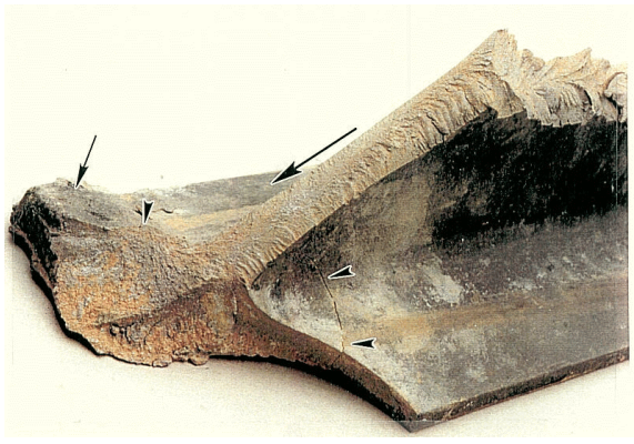
Photo 2. Top view showing thermite weld area, fracture initiation site, chevron markings, and other fracture locations
