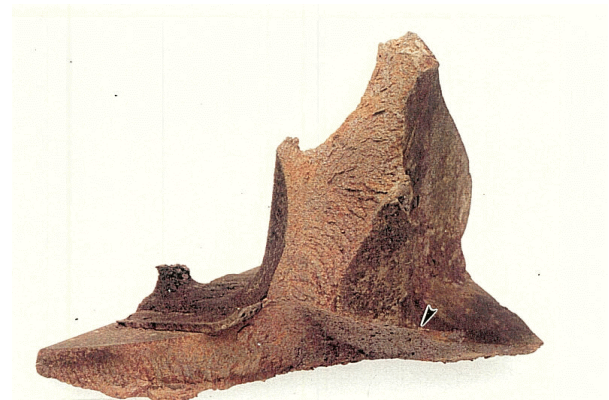
Photo 3. Mating piece of rail showing thermite weld area and fracture initiation location
