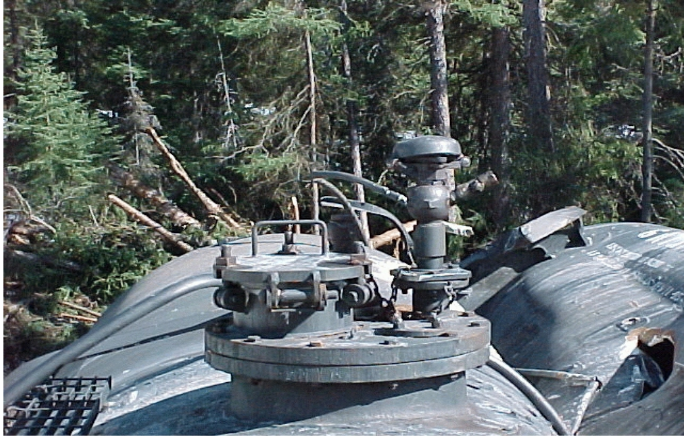
Figure 3 - A typical top fitting arrangement on a specification 111 tank car
