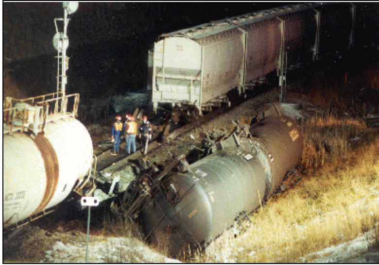
Figure 2 - Derailed tank cars overturned and resting in ditch.
