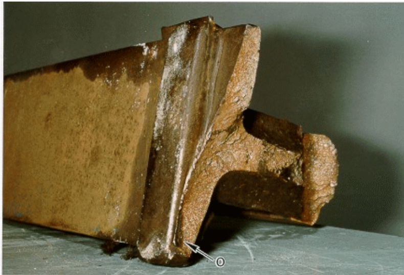
Figure 5—Location of pre-crack (O)
