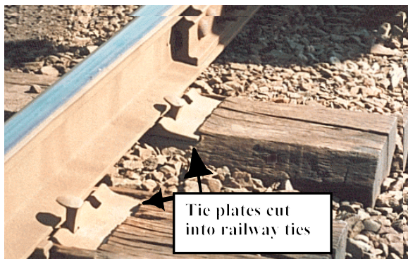
Photos 1 and 2. Track conditions near the initial point of derailment, including plate-cut ties and spikes.
