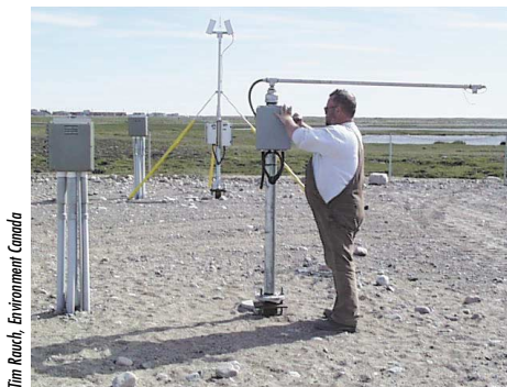
This snow depth sensor in Nunavut is part of a national network of climate observing stations stretching from coast to coast and into Canada's North.
