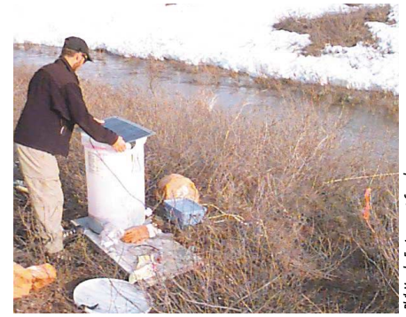
A researcher measures streamflow using dye injection techniques.
