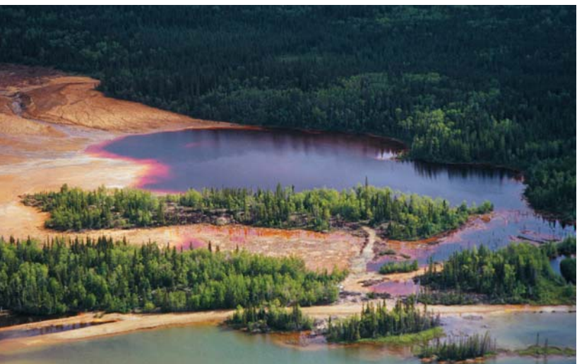
Low-quality drainage emanating from the Sherridon mine in northern Manitoba. At this site the wastes and workings have oxidized for over 70 years leading to the release of elevated concentrations of sulphide oxidation products to surface waters. The water quality is severely degraded in four lakes surrounding the mine. In the absence of an effective remedial program, low-quality drainage will continue to be generated for centuries. The volume of water impacted is many times the original volume of water consumed during the active stages of mining, suggesting that water audits for the mining industry require inclusion of consumption rates during both active and inactive stages of mining.
