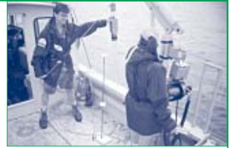
Scientists take sediment cores from the bottom of the St. Lawrence River to determine levels of trace metals in post-glacial marine clays exposed by decades of dredging.
