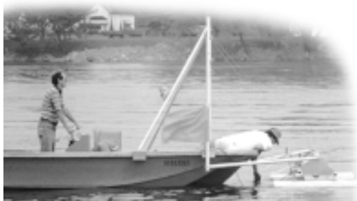
Sampling the surface microlayer of water for TBT
