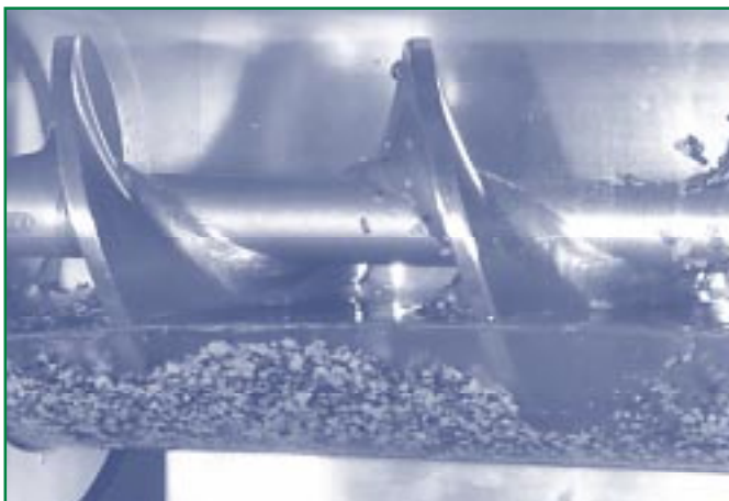
Canola flakes in hexane going through a processing system.
