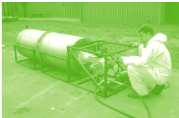
The portable burner developed by Environmental Technology Centre staff to flare waste fuel stored in remote locations.
