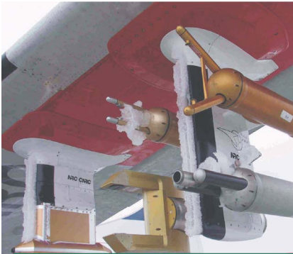
Icing that occurred on probes of the Convair-580 during a flight on February 19, 2003 at Mirabel airport in Quebec. The probes measure the size, shape and concentration of particles.
