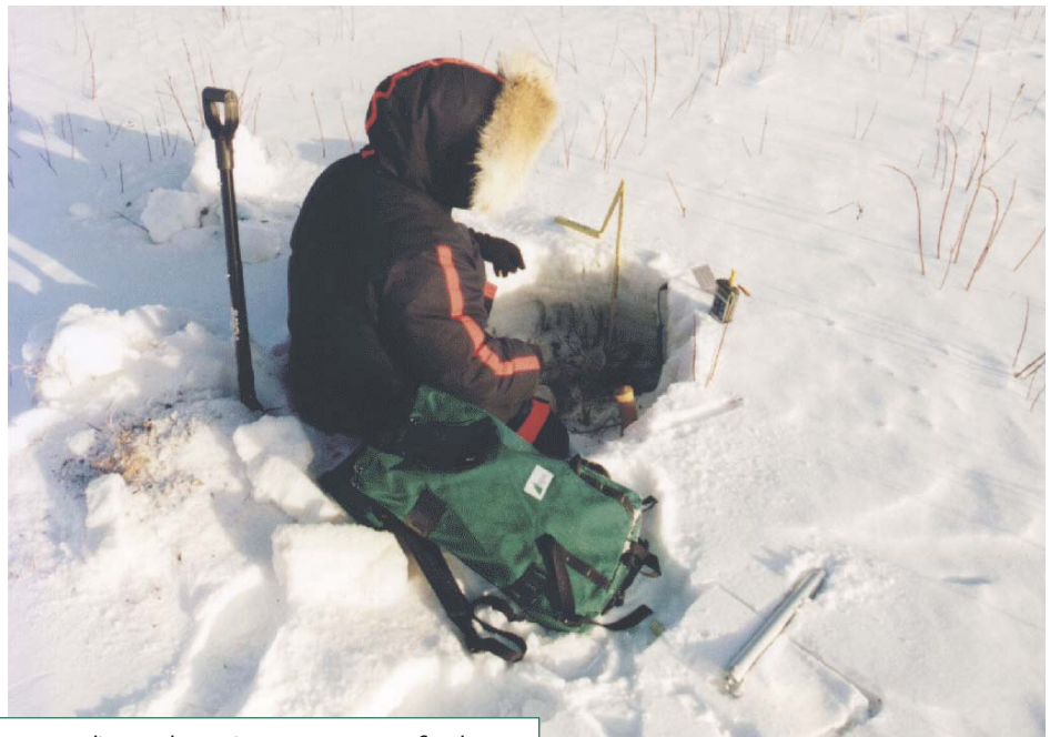
In-situ snow sampling to determine water content for the ground truthing of satellite measurements.
