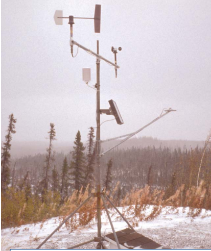
A portable meteorological tower at the Inuvik, NT, upper air site.
