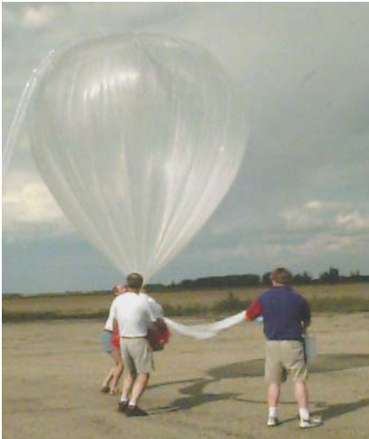
The Canadian ozonesonde network consists of six stations that launch ozonesonde carrying balloons weekly to determine long-term trends of ozone concentrations at all levels of the atmosphere.
