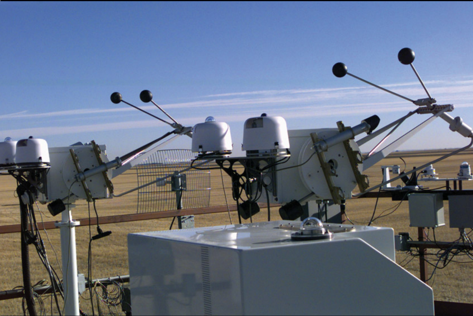
At the Bratt Lake Observatory, the Brewer spectrophotometer in the foreground measures ultraviolet radiation and the depth of the ozone layer while the solar trackers in the background measure diffuse solar radiation.
