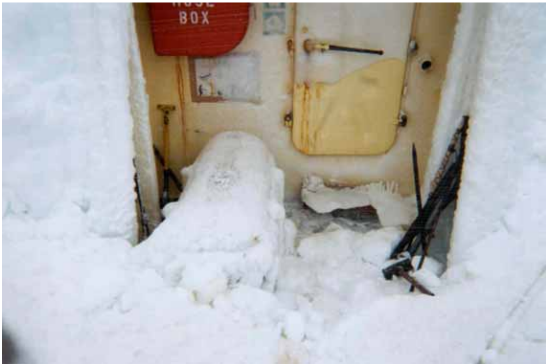
Figures 5.3D – Access to forecastle and forward liferaft severely hampered by presence of ice
