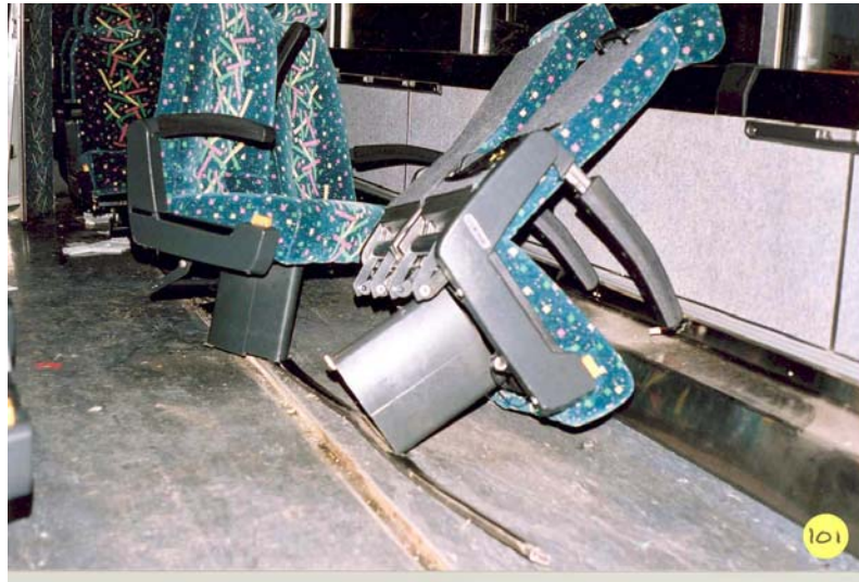
Figure 2: Case 4 - Example of Seat Detachment
