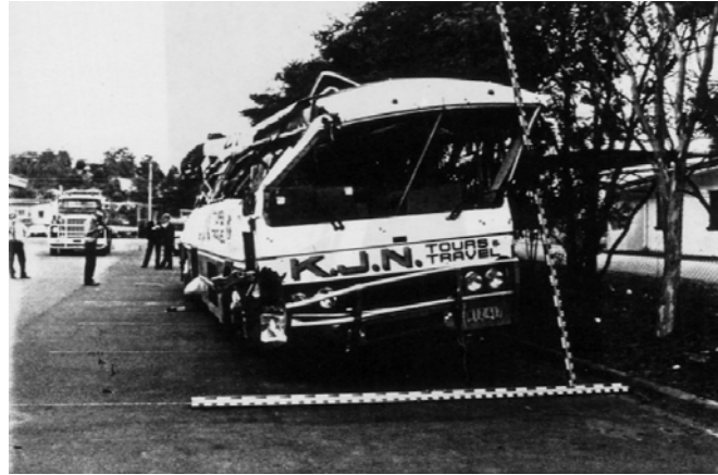
Figure 5: Front of the Bus in Case 4 Showing Deformation
