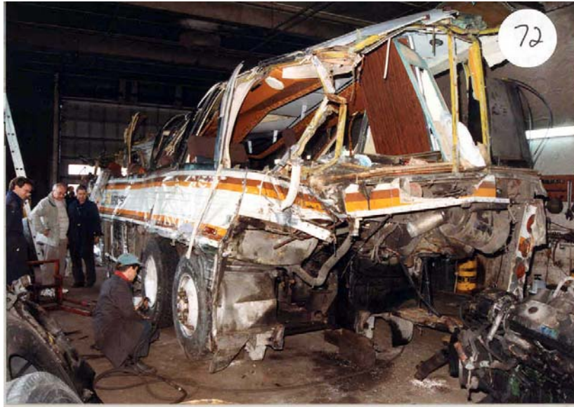
Figure 1: Case 1 - Left Rear View of Bus Showing Major Deformation
