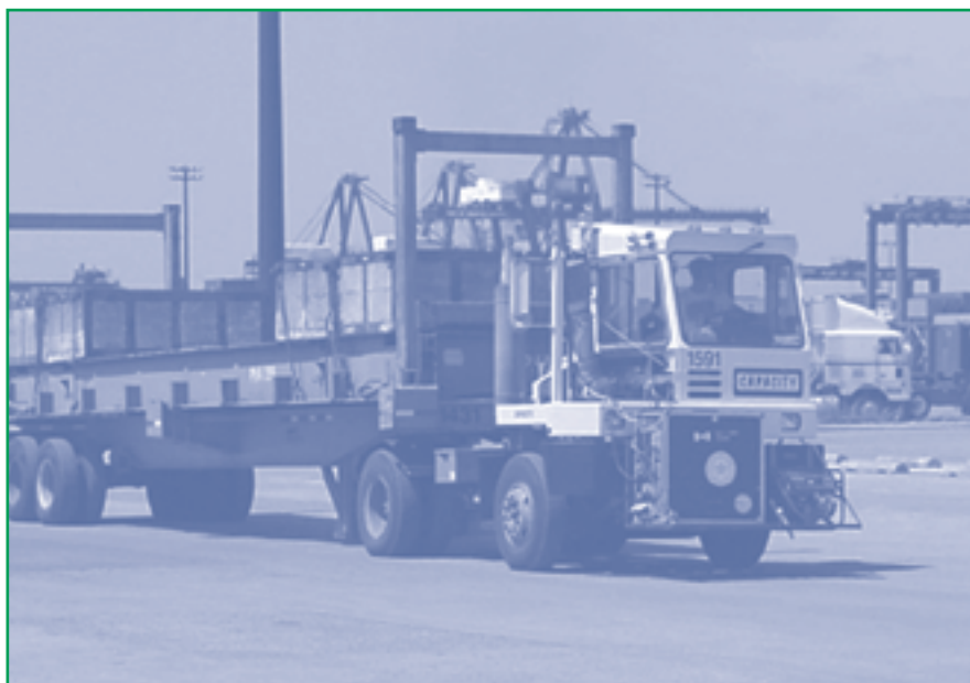
A DOES2™ portable emissions sampler mounted on a container hauler in the port of Houston, Texas.
