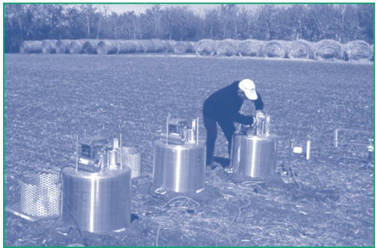
Placing flux chambers on a canola field to measure lindane volatilizing from treated seed.
