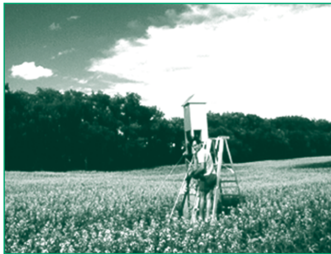
A high-volume air sampler measures concentrations of lindane and other airborne pollutants above a canola field in Saskatchewan.
