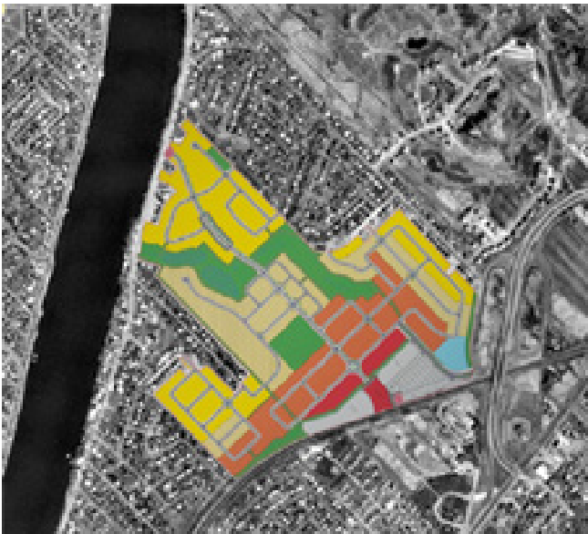
The 73-hectare site is located between the Richelieu River and the railway line. The high-density areas (red) are located near the station, and the outlying areas (yellow) are less dense. A primary school (blue) is also planned.
