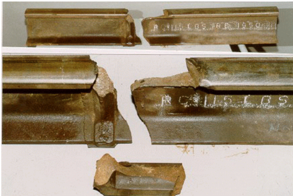
Figure 4 — Rupture du rail
