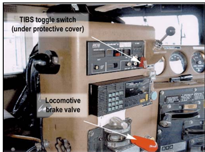
Photo 4. Locomotive control stand
