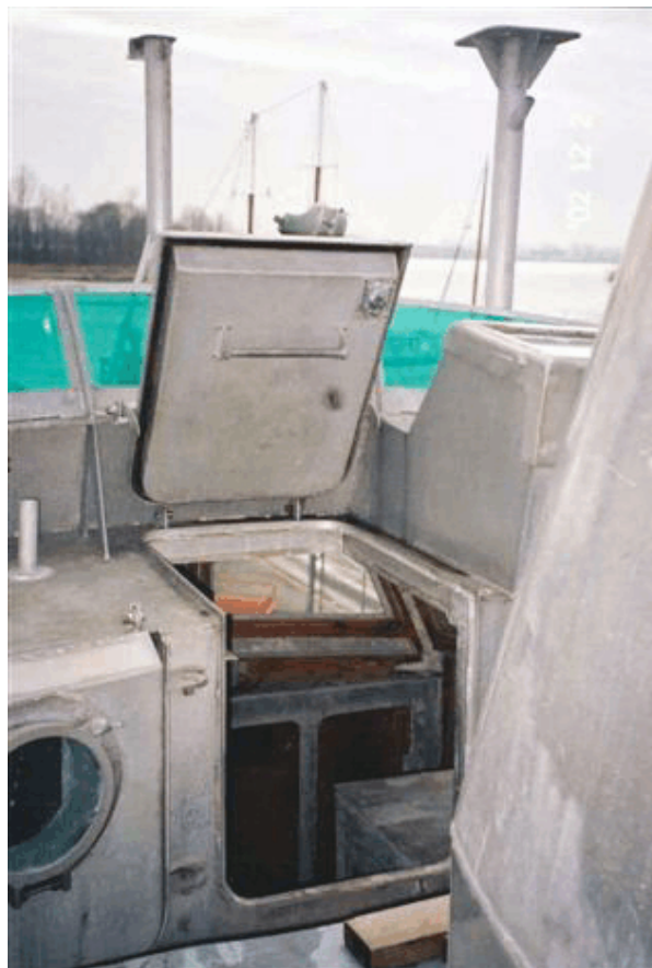
Photo 8. A combined hinged hatch cover and door on the centreline at the after end of the wheelhouse
