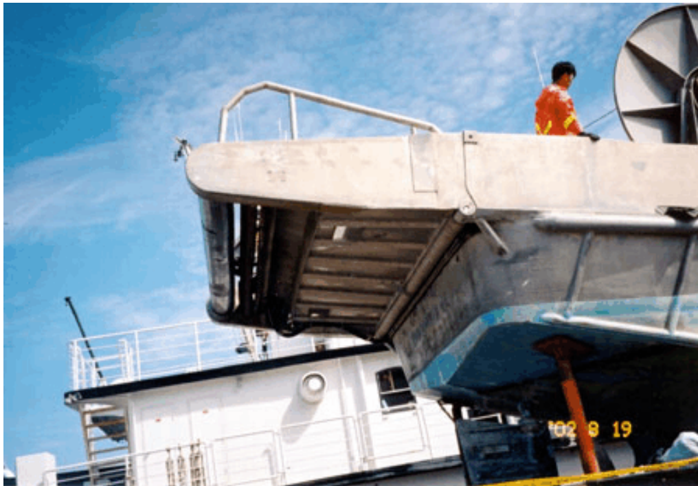
Photo 7. Stern of Cap Rouge II showing solidly constructed stern ramp extending beyond the transom. 19 August 2002
