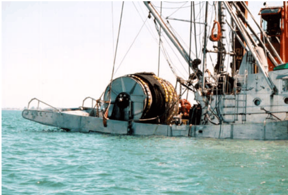
Photo 4. Working deck of Cap Rouge II showing west coast salmon seine net wrapped on net drum. 15 August 2002
