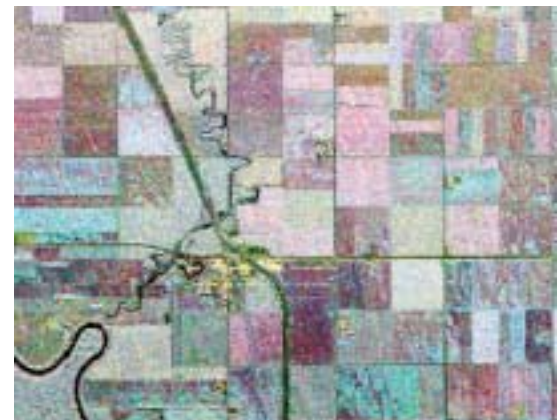
Colour composite image (HH, VV and HV polarizations) of agricultural fields in Southern Manitoba. (© CCRS. Acquired by CV-580 C-band SAR. Processed and provided by CCRS.)
