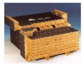
transponder traffic. Only those transponders carrying narrowband traffic are subchannelized. The sub-channels can have variable bandwidths on command, so that the payload can be configured optimally for the traffic patterns.
