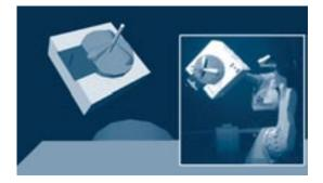
The ORPE Toolkit processes stereo camera images to compute 3D data and includes stereo vision systems, contains no moving parts, is of low power and survives well in the space environment. Pose (position and orientation) is estimated in near real-time from full resolution images on a PC system. The ORPE software toolkit can also integrate data from other 3D imaging systems such as range finders.
