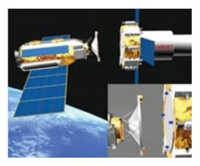
The CDT models the dynamics of contact as slightly resilient points of contact including friction, kinematic constraints and contact forces. It also includes precise geometry of the contacting
