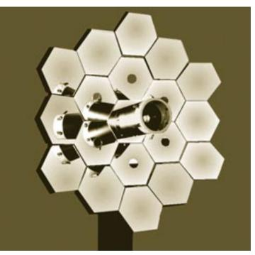
Through a CSA program, SensorTech has developed piezoelectric-based smart structures, a technology that allows lightweight structures to meet the challenge of maintaining their shape and resisting vibration.
