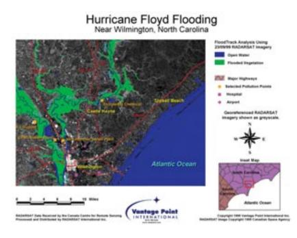
Monitoring Service, provides precise information on flood extent quickly, cost-effectively and conveniently. FloodTrack technology distinguishes between open water and flooded vegetation with high precision and provides fully georeferenced flood contour maps that can be delivered via the Internet.
