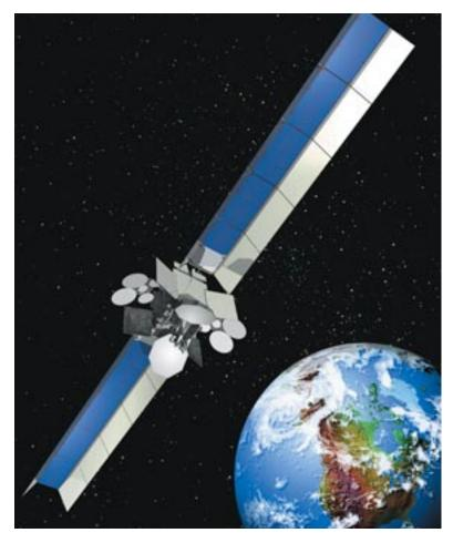
To overcome the performance limitations of multiple beam antennas using a single element per beam, EMS Technologies devised high-directivity efficiency feed elements for high-frequency multibeam reflector antennas. The innovative feed element technology developed, with funding from the CSA, allows for significant RF (Radio Frequency) performance improvement, notably on gain and sidelobe isolation.
