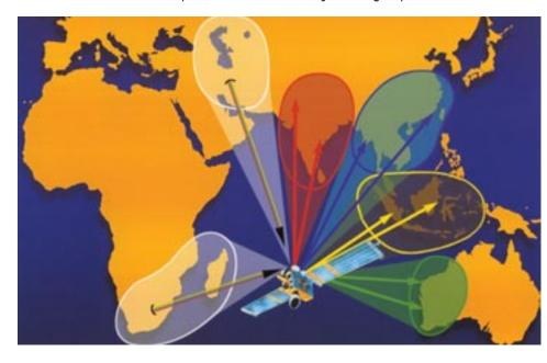
BEAM\*LINK<sup>™</sup> offers vastly increased traffic management flexibility for multi-beam satellites, increasing service provider revenues up to \$40 million per year, and enabling the introduction of new services. This technology will fly on the next generation Anik F2 satellites. COM DEV's recognized leadership in this technology sector has lead to a contract award to build a Ka-band processor for the ASTRA 1K satellite, which will provide two-way Internet via satellite in Europe.
