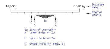
To test a scale using error weights, it is necessary to know "where you are" within a scale interval (to have a reference point). The zero reference point is the point within the zero interval at which the scale is located when under zero load. It is necessary to establish the true "zero reference point" location in order to determine the relative location of the ZU within the interval.
