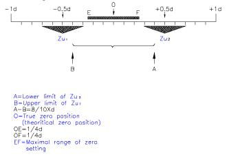
If the zero reference point is not located at mid distance of the interval (equidistant from  $ZU_1$  and  $ZU_2$ ), any deviation must be taken into consideration in the calculation of internal or true errors.
