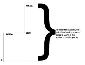
The possible adjustment of the IZSM of a separately approved indicating element must not exceed 20% of the maximum approved capacity of the indicating element, because the performance of the load receiving/weighing elements to which it will be associated is not known.
