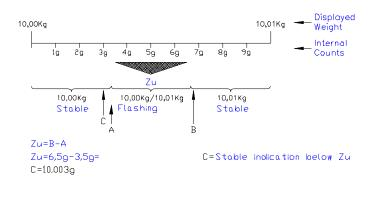
**Note:** On a multiple range device and a multi-interval device the determination of the location and the width of ZU must be done for each range.
